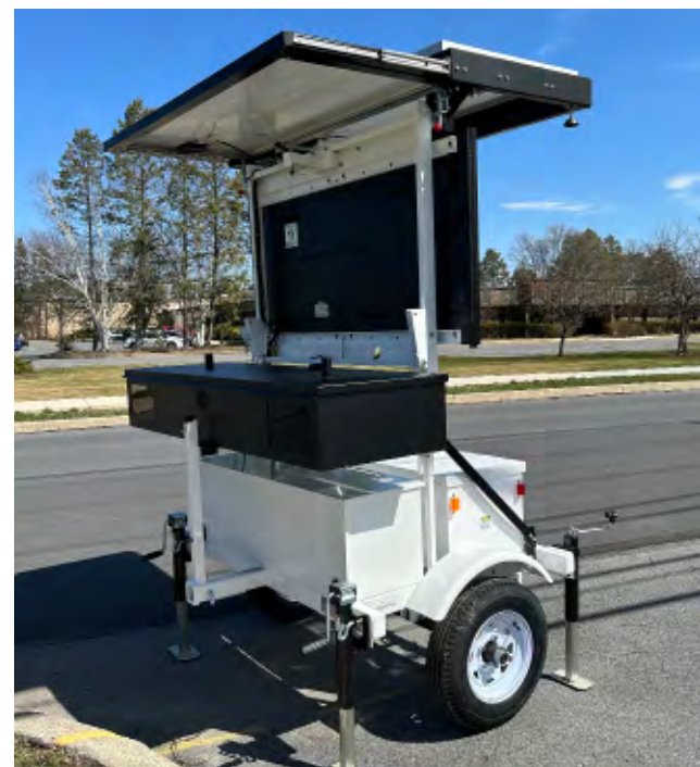
SpeedAlert 24 radar message sign on 380W LPR camera-ready trailer with two-camera enclosure box
