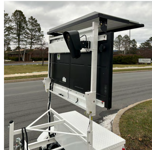
190W LPR camera-ready trailer with cameras attached to mounting plate
