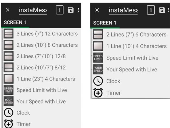
**TIP:** For SpeedAlerts, the **Your Speed with Live** and **Speed Limit with Live** templates are particularly useful in creating radar-based messages. They include the layout shown below, with programmed placeholders to display the speed limit you set up for the sign and radar-detected speeds.
