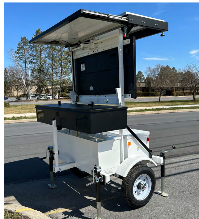
SpeedAlert 24 radar message sign on 380 LPR camera-ready trailer with two-camera enclosure box
