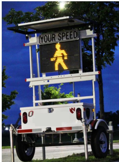
*[Figure 1] ATS 5 Trailer and SpeedAlert radar-enabled messaging sign*
