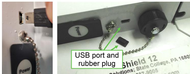
[Figure 4] USB port on Shields, SA 18s, and IA 18s
