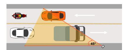
If you use a smaller horizontal angle than 45 degrees (more directly facing the traffic), speed data will be improved, but vehicle counts will not be as accurate.
