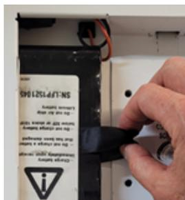
*[Figure 1] Slide the battery*
