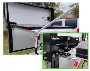
CAUTION: As you raise the upper frame, be careful and use both hands, moving the handle slowly and applying counter weight. The load will shift as it nears the final position.
