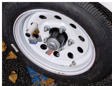
[Figure 17] The axle lock bar - locking end
