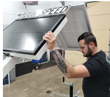
[Figure 4] Unfolding the trailer mast
