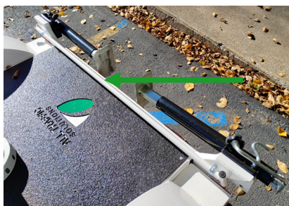
[Figure 14] Axle lock bar stowed
