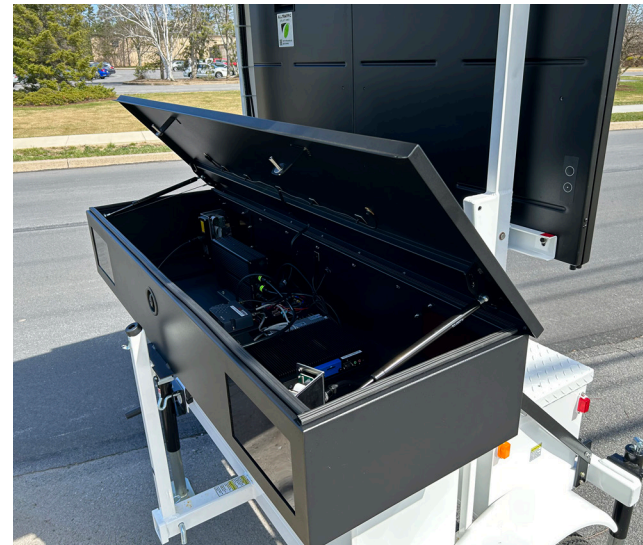
Open two-camera enclosure with cameras installed
