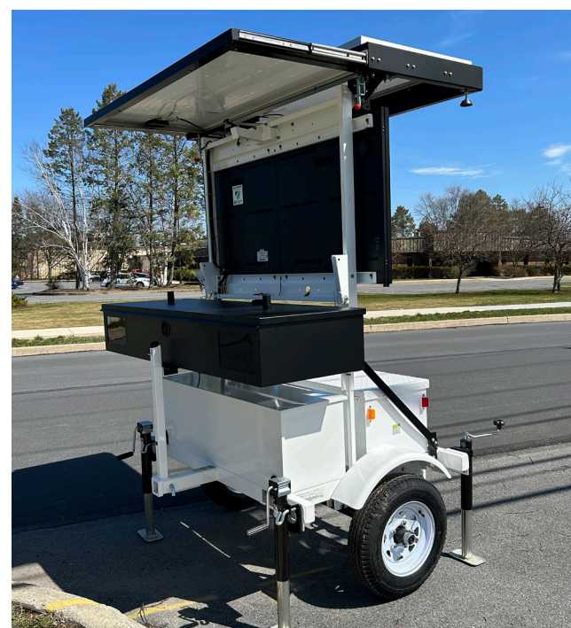
SpeedAlert 24 radar message sign on 380 ALPR camera-ready trailer with two-camera enclosure
