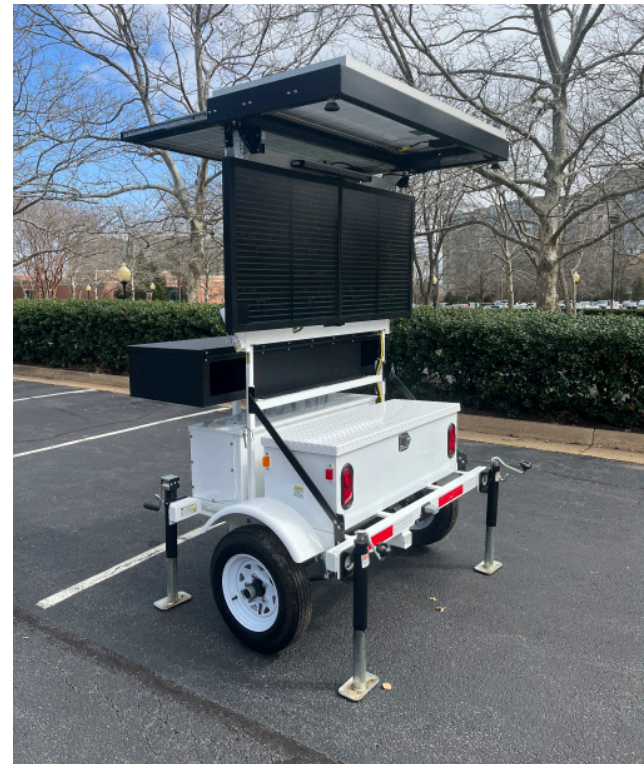
SpeedAlert 24 radar message sign on 380 ALPR camera-ready trailer with two-camera enclosure
