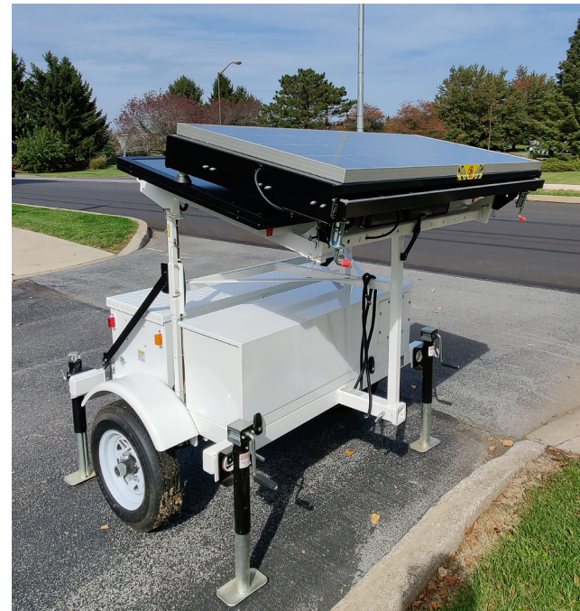
SpeedAlert 24 radar message sign folded down on 380 ALPR camera-ready trailer
