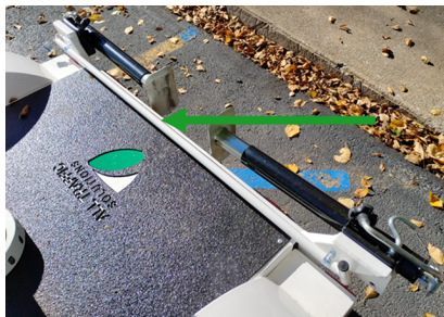
[Figure 13] Axle lock bar stowed
