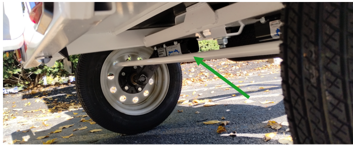
[Figure 12] The axle lock bar installed
