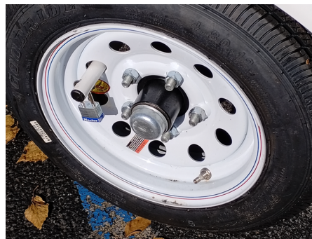
[Figure 16] The axle lock bar - locking end
