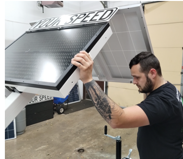
[Figure 4] Unfolding the trailer mast
