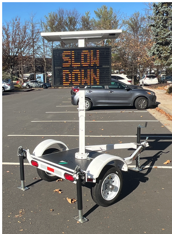
[Figure 1] ATS 3 Trailer and SA 18 with Integrated Solar
