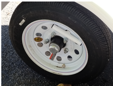
[Figure 15] The axle lock bar - T-bar end
