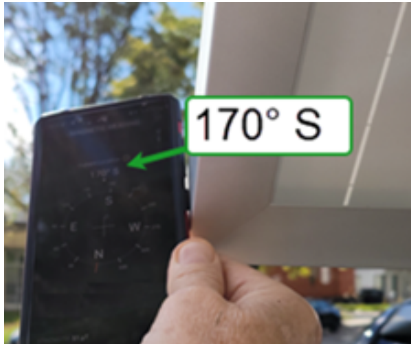
[Figure 13] Aiming the panel to True South with a compass app
