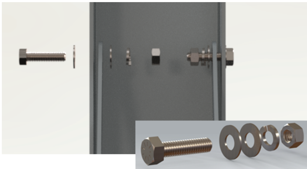
[Figure 5] Exploded view of the nuts and bolts
