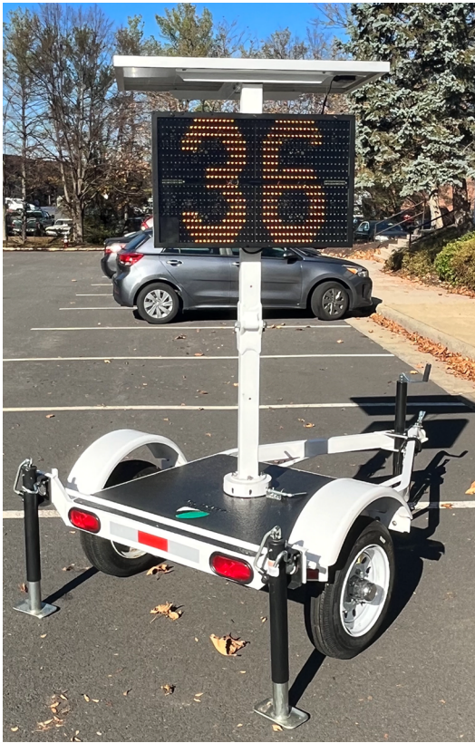
[Figure 1] ATS 3 Trailer with a SpeedAlert 18 Radar Message Sign and solar panel
