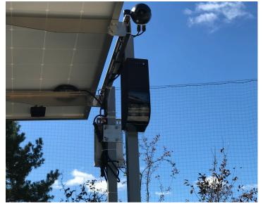
Sign can display numeric values as well as OPEN, FULL, and CLSd with super-bright wide viewing angle LEDs.
