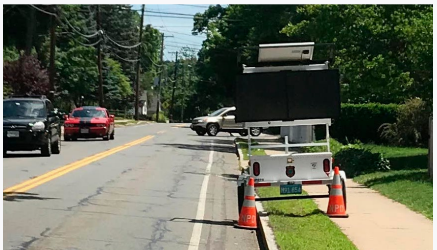
A SpeedAlert 24 on an ATS 5 Trailer stationed on a residential Natick street in response to a speeding complaint
