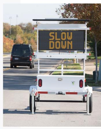
An InstAlert 24 variable message sign mounted on an ATS 5 trailer is an effective and portable traffic calming method. Messages can be changed remotely and the trailer can be equipped with ALPR for additional enforcement capability.
