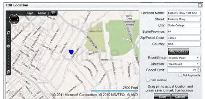
*Not Applicable* can be checked if the sign has no radar or there is no speed limit at the location.
