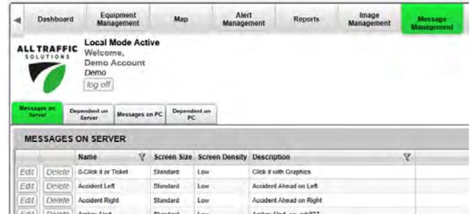
Messages are single, three screen messages. Dependent Messages are groups of five messages with a specific message displayed related to a specific vehicle's speed relative to the speed limit.
