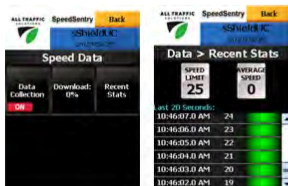
Click on the *Download* button to download data to the PDA. Once downloaded you can tell the PDA to erase the data file on the speed display. The *Download* button indicates how full the memory is. The *Recent Stats* shows the last 20 seconds of readings and will update continuously when you are connected to a sign.
