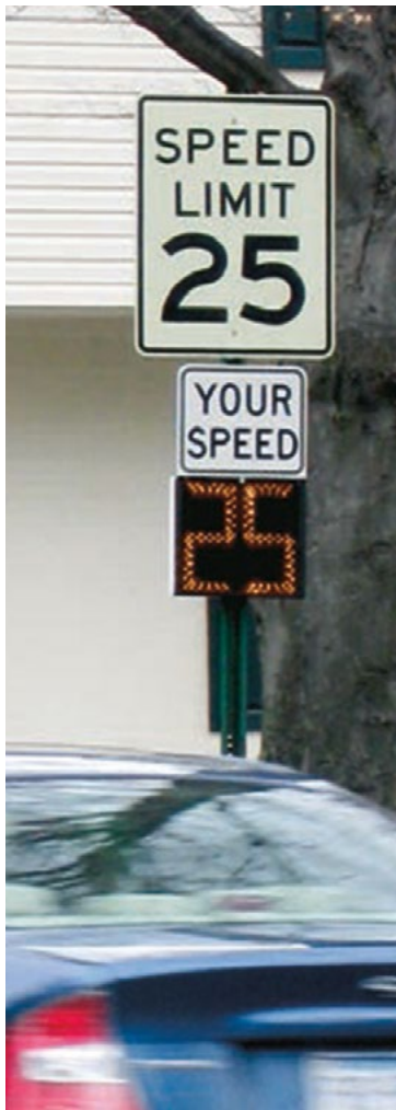
A Shield radar speed sign installed below the speed limit sign reminds drivers to slow down.
