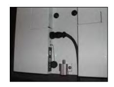
The Shield 15 uses screws to attach the unit directly to the trailer. The mounting bracket is not required. The on-board control buttons for speed and mode time out after 5 minutes of inactivity to prevent tampering. To reactivate control turn the unit off and on again and they will work until inactive for 5 minutes.
